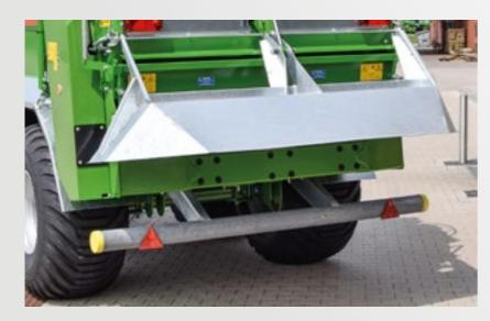
The optional, hydraulically operated **spread pattern limiter** prevents the contamination of roads, paths and waterways etc. and ensures precise and uniform spreading of fields, right up to the edges.
