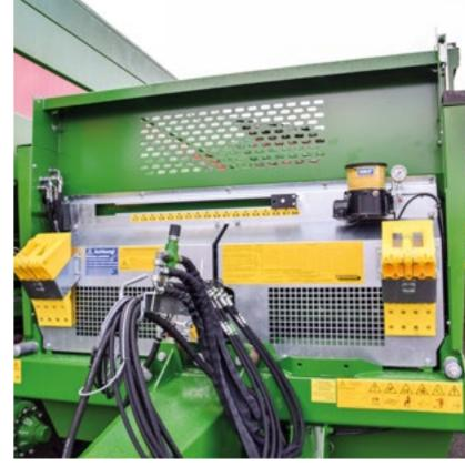
Exact height indicator for the optional hydraulic dosing wall.
