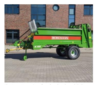
The **M 1080 Manure Spreader** with a robust chassis, bolted drawbar and sturdy jack stand for large payloads. A one-sided wall attachment for increasing the load volume is optionally available.
