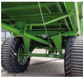
The **self supporting bin** eliminates the need for a supporting frame and thus offers almost no possibilities for dirt to collect. Both result in minimum maintenance and cleaning times.
