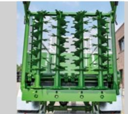
M 2120 SW E/T SW spreader unit with 1,300 mm throughput. Four vertical beaters with bolted flat steel tines.
