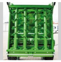
M 2120 SX E / T SX spreader unit with 1,400 mm throughput. Four vertical reinforced beaters with bolted flat steel tines.
