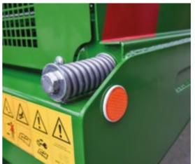
With the automatic tensioning system, which is visible from the tractor, the four high-strength scraper floor chains can be easily adjusted from the front. This allows for a high degree of safety and smooth operation.
