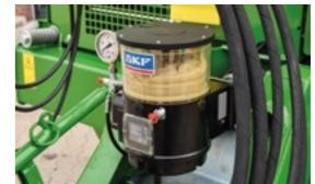
The optional central lubricating system provides for a continuous flow of lubricant which is adapted for each individual bearing. This significantly reduces maintenance efforts.
