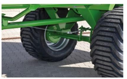
Wide tires with low tire pressure prevent soil compaction.
