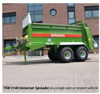
**Optional high or low drawbar** with fold-up jack stand. "Jost" landing gear for easy coupling as standard equipment. The side wall height - and thus the load capacity – can be increased using **side wall extensions.**
