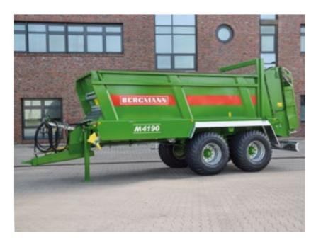
**Optional high or low drawbar** with spring-mounted drawbar for high driving comfort and good driving stability. The use of spacers makes it possible to ideally adjust the **drawbar height** for every tractor.
