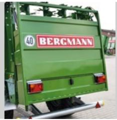
Hydraulically operated **spreader unit hood.**
