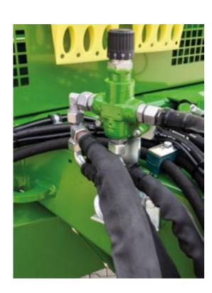
The optional **manual scraper floor control** makes exact material dosing possible.
