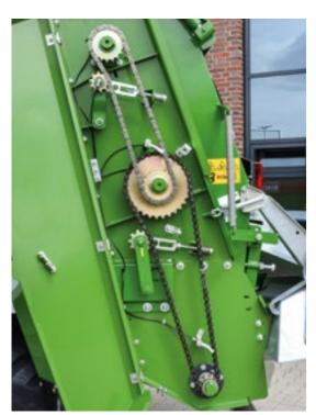
TSW spreader unit drive via roller chain.
