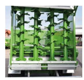
**Spreader unit SZ** 1,400 mm throughput. Four vertical beaters with bolted flat steel tines and hydraulically operated spreader unit hood. The spreader unit is driven via transfer case and four roller gearboxes.
