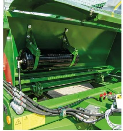
The large front wall **maintenance hood** provides for easy cleaning and maintenance of the scraper floor, which can be easily seen through the window.
