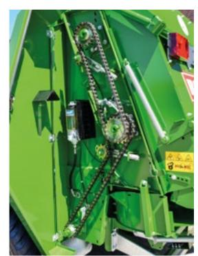
TSW spreader unit drive via roller chain. Spring-mounted chain tensioners ensure optimum power transmission and low
