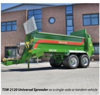
**Optional high or low drawbar** with fold-up jack stand. "Jost" landing gear for easy coupling optionally available. The side wall height and thus the load capacity - can be increased using **side wall extensions.**
