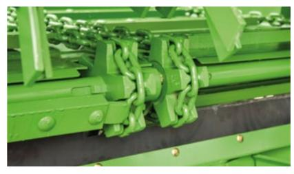
The hydraulic scraper floor drive with spur gear box ensures safe transport of the most diverse materials to the spreader unit.
