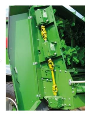
SZ spreader unit 1,400 mm throughput. Four vertical beaters with bolted flat steel tines.
