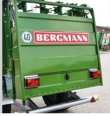
Hydraulically operated **spreader unit hood**
