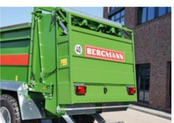
Hydraulically operated spreader unit hood.
